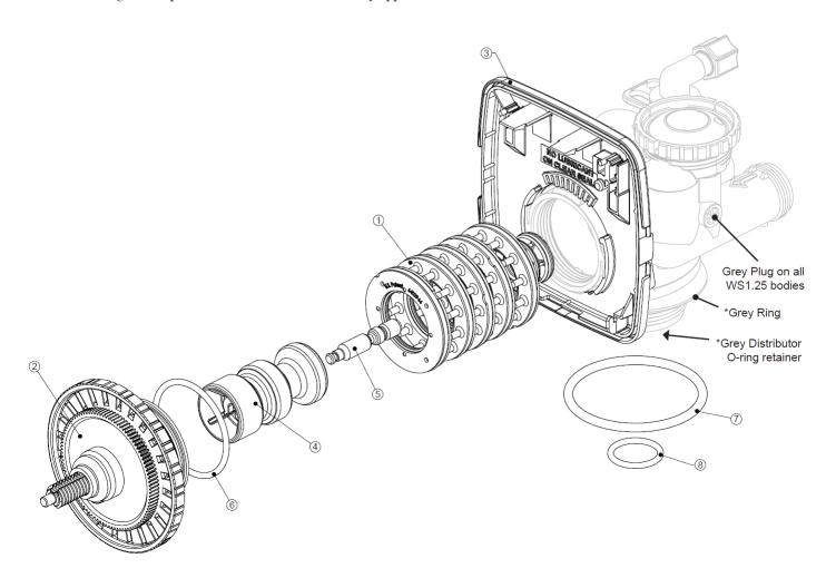
Injector Cap, Injector Screen, Injector, Plug and O-Ring
