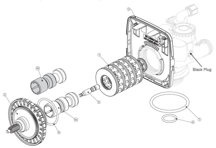
WS1.25 Drive Cap Assembly, Downflow Piston, Regenerant Piston and Spacer Stack Assembly
