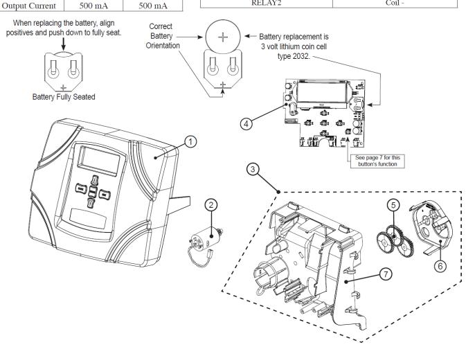
WS1 Drive Cap Assembly, Downflow Piston, Upflow Piston, Regenerant Piston and Spacer Stack Assembly
